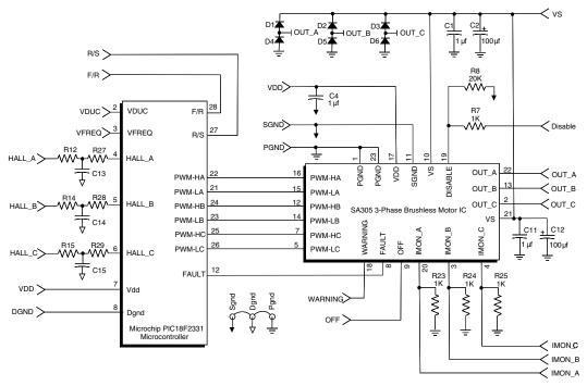
A specific example - Combining the SA305 Brushless Motor IC with a Microchip PIC18F2331 Microcontroller
