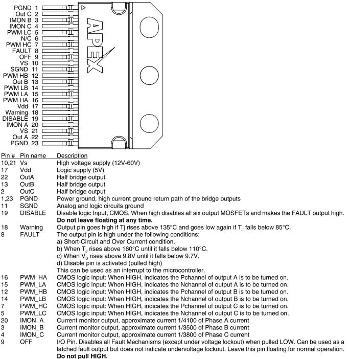
All inputs are CMOS levels. Inputs can accept CMOS levels as low as 3.3 volts. CMOS logic inputs cannot be left floating at any time.
